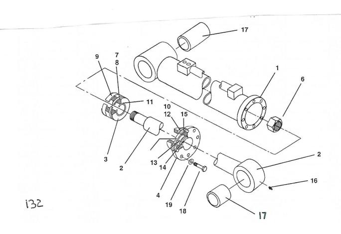
Grapple Cylinder P/N: 46556B replaces 18332B Cylinder Assy.
