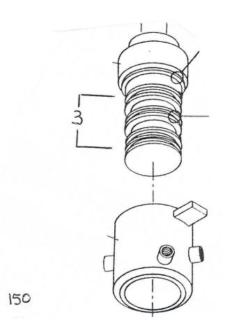
Rotary Manifold Assy P/N: 17609B replaces 7374B and 10459B Rotary Manifolds.
