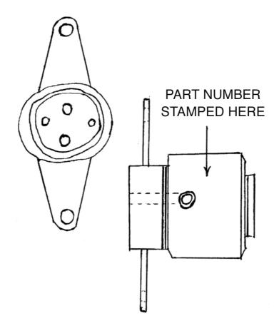
PR10048869 Swivel Assembly- 2 Circuit
